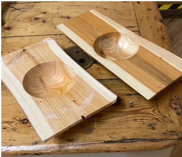
Round-bottomed winged bowls. The front one was turned on the night but remains to be finished, with the wing ends trimmed off.
